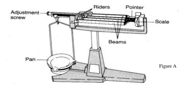
When the balance is required for determining mass, you will use a balance like the one shown in Figure A above. The balance has a readability of 0.001 g. This means that your mass readings should all be recorded to the nearest 0.001 g.
