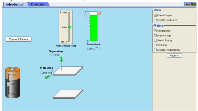
a) Vary the area of the plates. How does the Capacitance vary with area A? Show your calculations below
